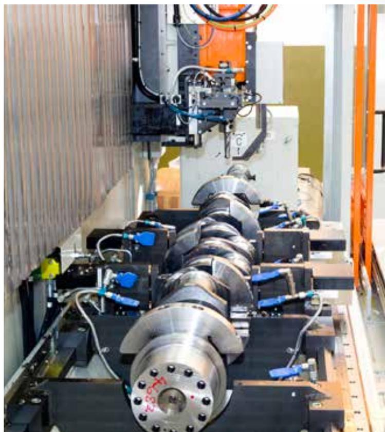
Version for balancing large shafts with the main journals supported on sleeve bearings; includes high capacity correction unit, complete with clamping, drill thrust back-up and features automatic tool change for deburr procedure.
