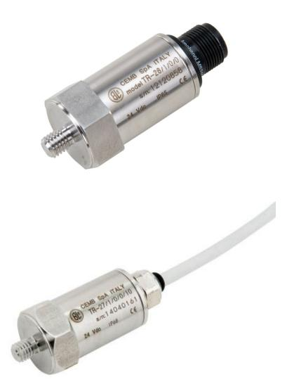
This transmitter can provide an electrical signal directly proportional to the vibration of the point to which it is fastened, with direct interface to an acquisition system made in 2-wire technique (4-20 mA current loop).
