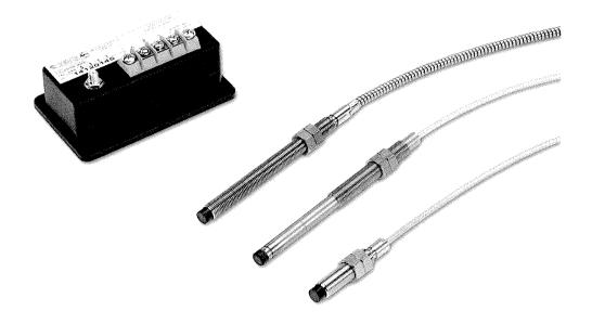
The T-NC/8-API converter, together with ST-NC/8 sensor and CPT-NC/8 cable, measures the relative vibrations or axial displacement of a shaft with respect to a support. The output is a negative voltage value proportional to the target distance.
