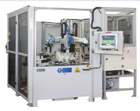
Three station balancing isle for automotive electric motors where the first station is a loading/unloading spot where the rotor is placed either manually or through a robot.
