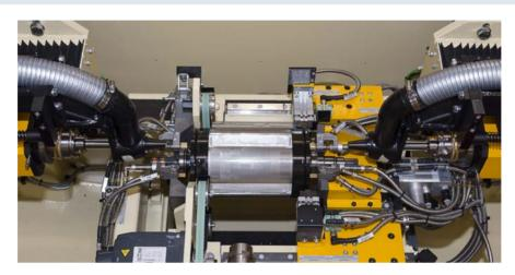
Balancing system composed of robot cell with two balancing machines, each one with unbalance measurement and correction function. The anthropomorphic robot loads and unloads the pieces from the client's pallet line on the balancing machines and can also load the master rotors from internal stores.
