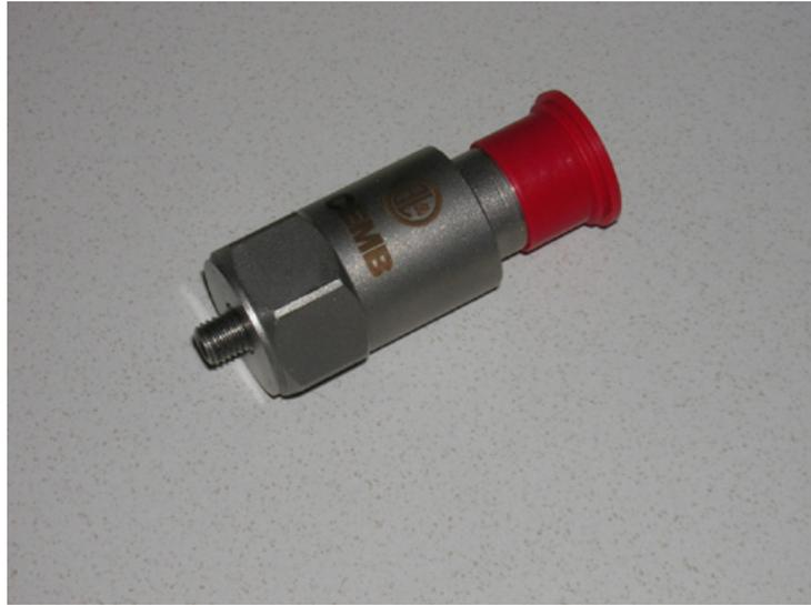
The model TV22 seismic transducer measure the absolute vibration of the machine by the securely mounted to a flat surface. It supplies an output signal directly proportional to the speed of vibration of the point to which it is fastened. Such signal should subsequently be processed by one of the measuring channel of a serial "T" processing unit.
